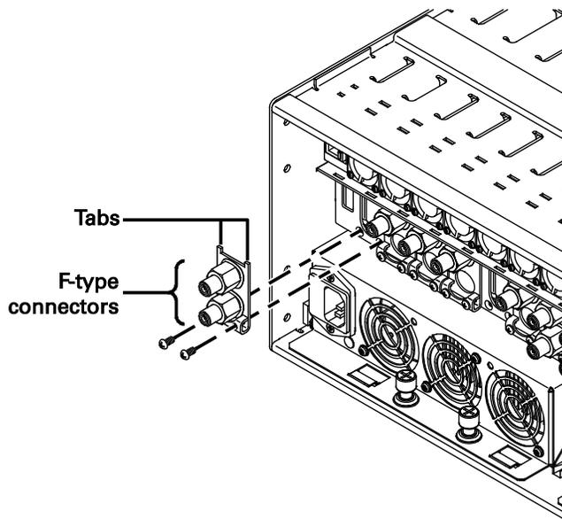
**Figure 8: Installing the RF interface connectors on the rear of the GX2-HSG\***
