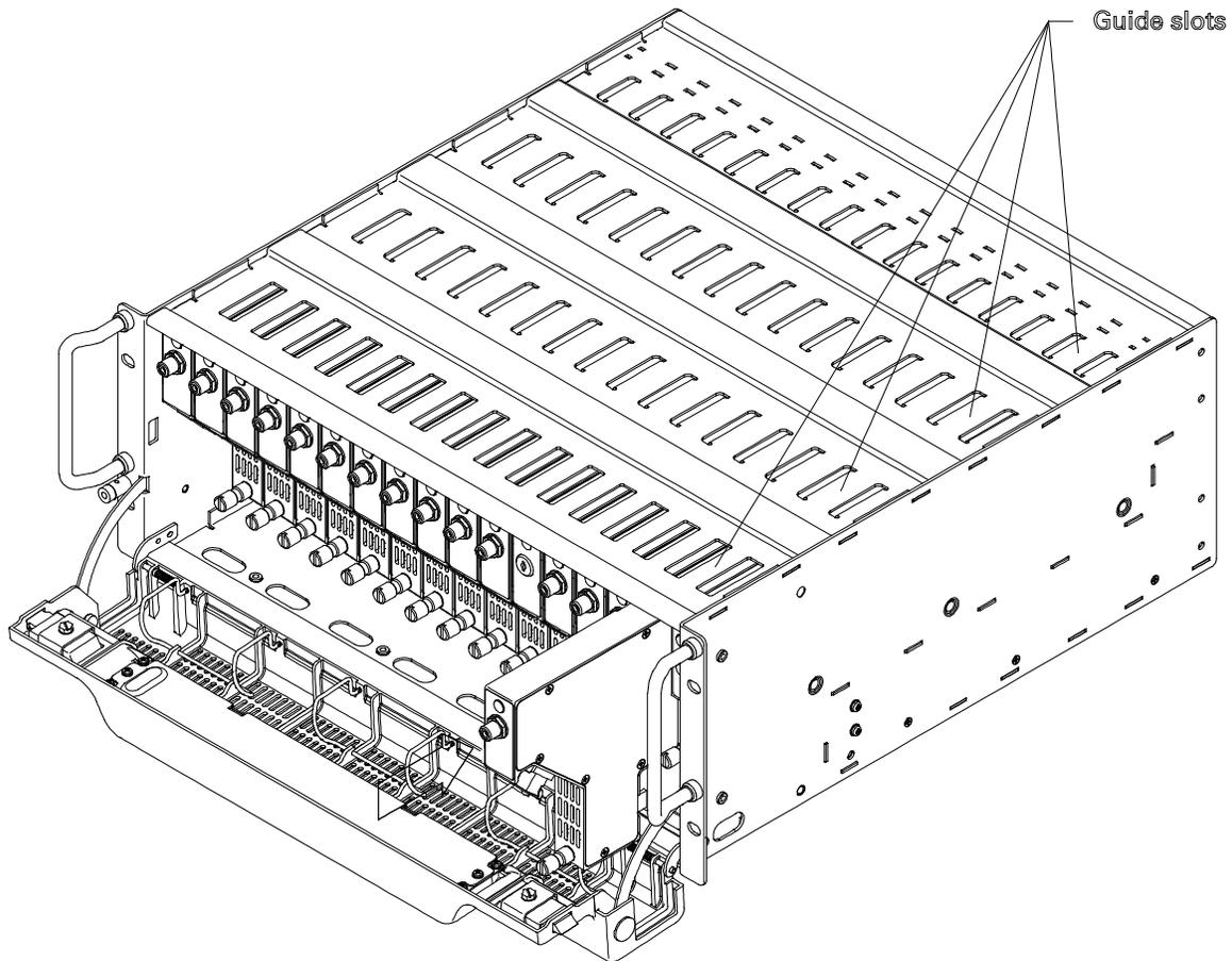
**Figure 14: Inserting the GX2-EA1000C\*/\* in the GX2-HSG\***
