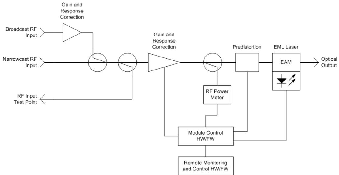
**Figure 4: GX2-EA1000C\*/\* Block Diagram**
