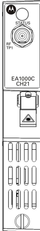
**Figure 6: GX2-EA1000C\*/\*front panel**
