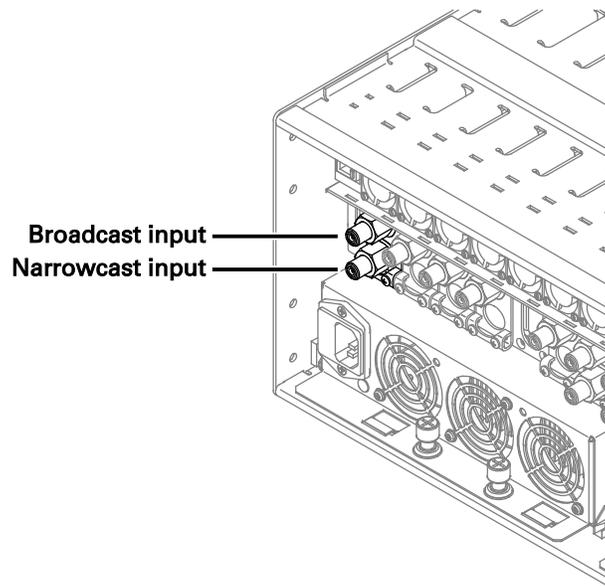
**Figure 15: GX2-HSG\*rear-panel RF connections**
