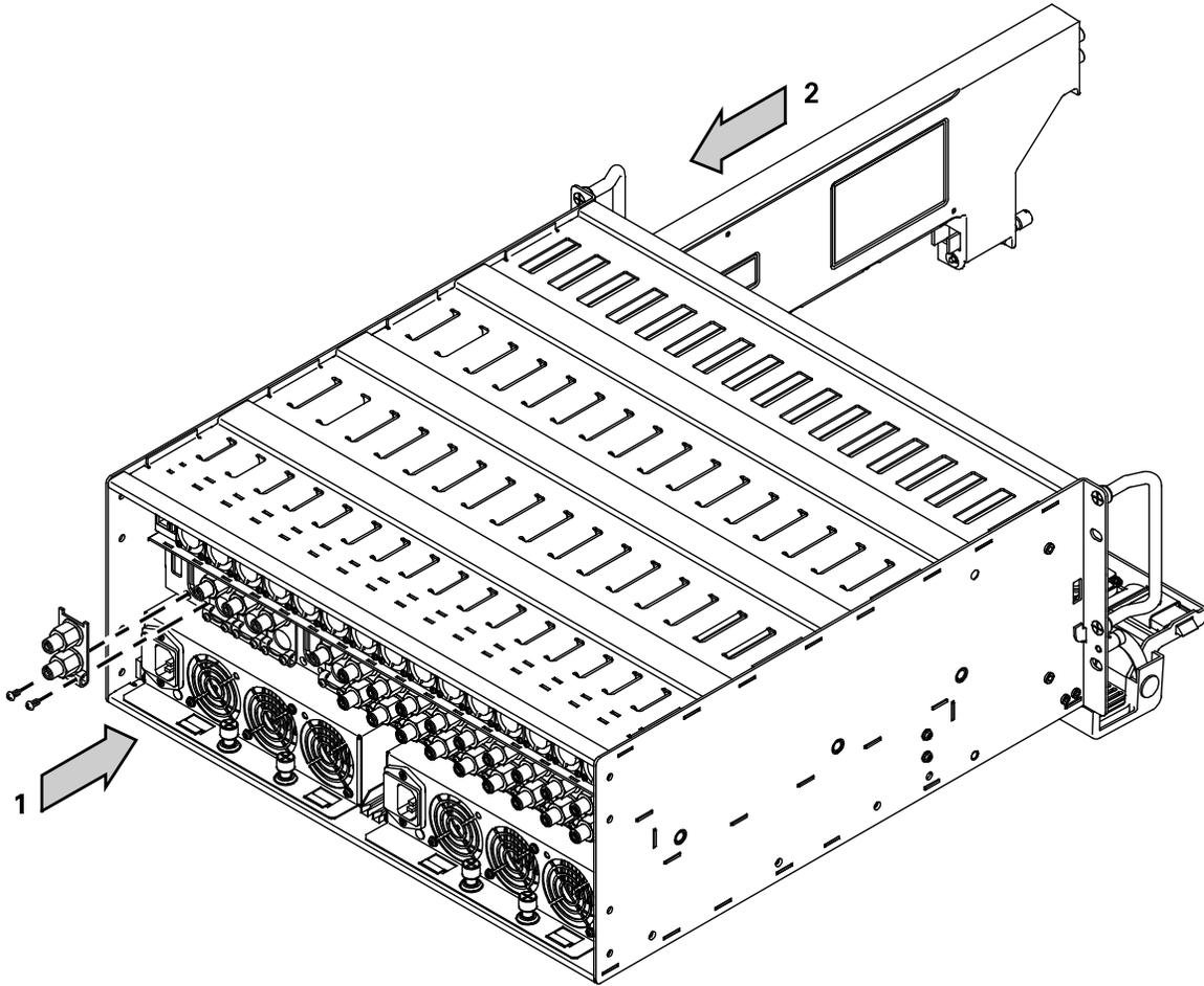
**Figure 13: GX2-EA1000C\*/\* installation in a GX2-HSG\***
