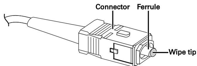
**Figure 10: Cleaning the SC/APC connector tip**
