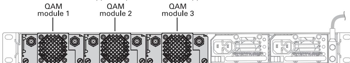
Each QAM module has two RF output ports, each of which supports either four or eight adjacent QAM carriers. The 2x4 QAM modules support up to four QAMs per port and the 2x8 QAM modules support up to eight QAMs per port, allowing the following configurations:
