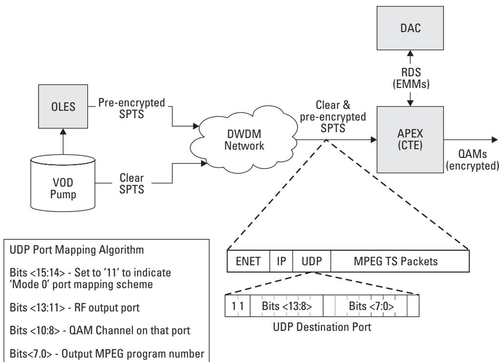
*Note: The figure above shows the standardized port mapping mode as defined by Harmonic. While other schemes have been used (and were supported by the SEM), the APEX1000 will only support this exact scheme.*
