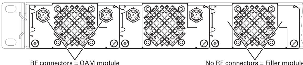
*Note: When viewed from the back of the unit, #1 is the left QAM module, #2 is located in the middle, and #3 is located on the right.*
