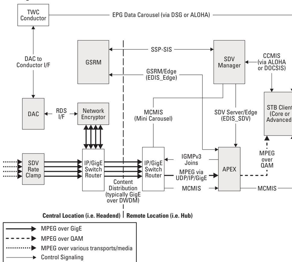
Note: Shown with Motorola components, as well as the Time Warner Conductor required to support the TWC guide/SDV client (MDN/ODN) running in the set-top.
