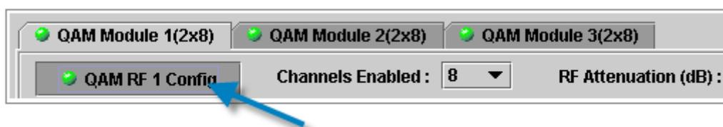
Figure 6-13 — QAM RF Port Configuration
