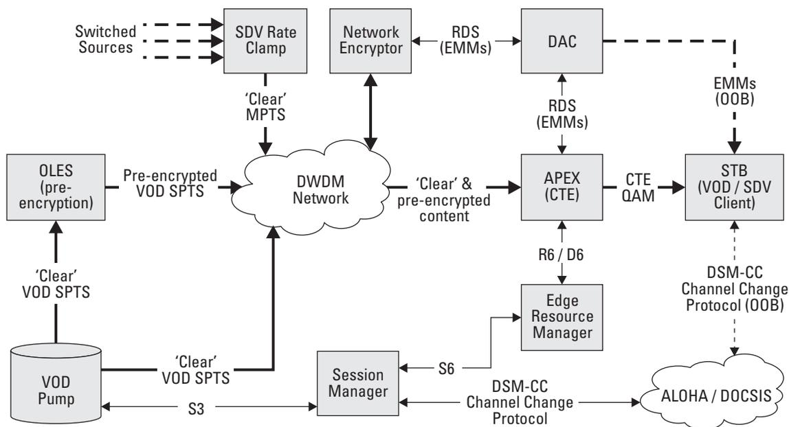
*Note: Multiple encryption paths are possible using an OLES, the Network Encryptor, or the APEX1000 itself.*
