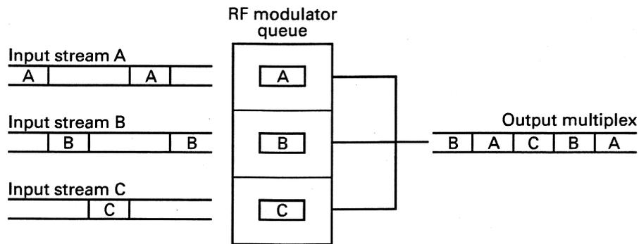
The multiplexer then builds the output multiplex for the RF modulator by extracting packets from each buffer in the RF modulator queue in sequence (that is, one packet from the A buffer, one from the B buffer, one from the C buffer, and so on).
