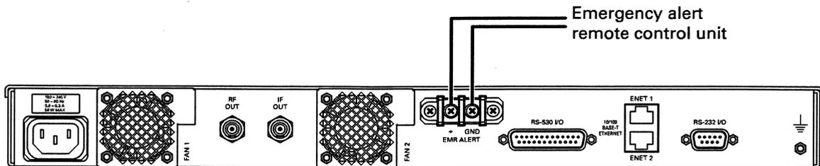
2. Align and then secure the ground wire to the alert connector (labeled  $\perp$ ) on the back of the unit.
