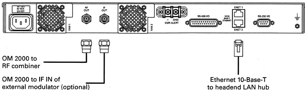
To connect the Ethernet and RF-modulator output cables:
