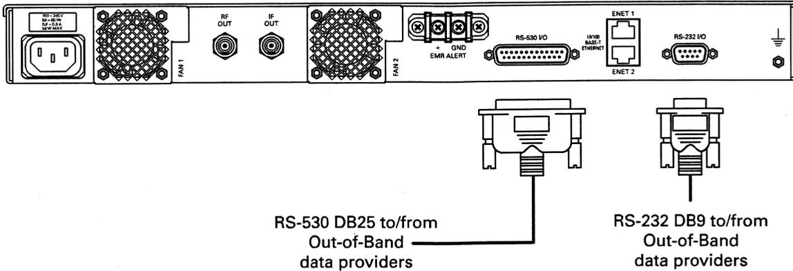
2. Push the cable in until the connector is fully engaged. Do not bend the pins.
