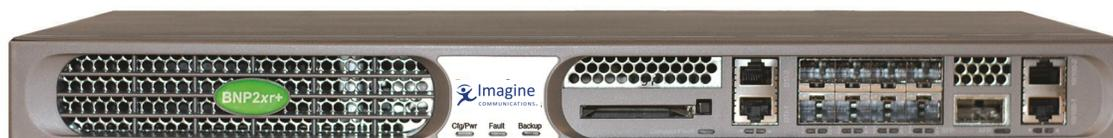
Receiving input through its Gigabit Ethernet or ASI interfaces, the BNP can statistically multiplex while performing grooming and digital ad and overlay insertion.
