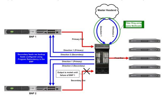
This configuration illustrates a single Headend with one Switch using Fiber Ring Redundancy.
