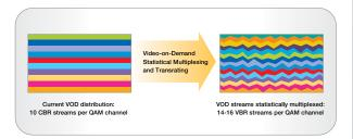
With the addition of the RGB DBM, operators can take advantage of bandwidth savings of 50% or more by statistically multiplexing approximately 15 programs within a single MPTS transport, while still maintaining optimum picture quality. This additional bandwidth can be used to introduce or increase the number of on-demand high definition (HD) VOD programs offered, or can be used for other bandwidth-hungry applications such as high-speed Internet.
