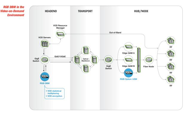
QAM channels. Although this conversion simplifies the allocation of the video programs, it also lowers the overall efficiency of the SDV architecture, and can result in lower quality video programs. RGB's DBM offers a plug-and-play solution for SDV allowing the delivery of the video programs in their original and native VBR format, while optimizing the bandwidth and improving the video quality.
