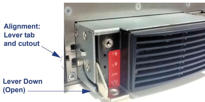
2. Guide the power supply unit into a slot, at the chassis front power bay, until it stops.
