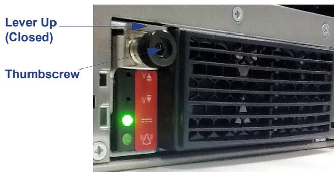
4. Insert the thumb screw and turn clockwise to tighten it.
