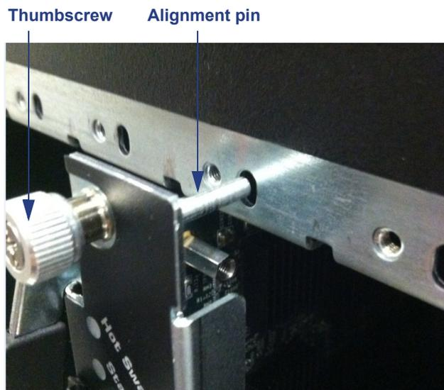
3. After pressing the card into the backplane, press the ejector handles down to the faceplate, to set each in closed position.
