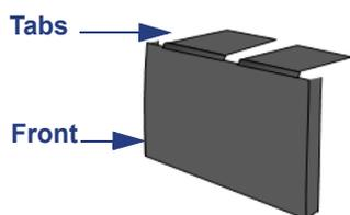
When placed in this position at the terminal block, the connected cables are guided out of the bottom edge.
