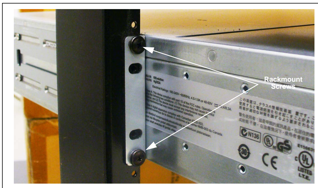
Figure 2.16 - Securing Front Bracket to Rack
