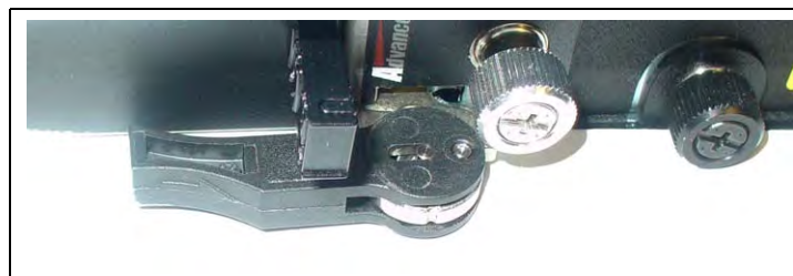
Figure C.25 - G10 IIC Ejector Handle Closed
