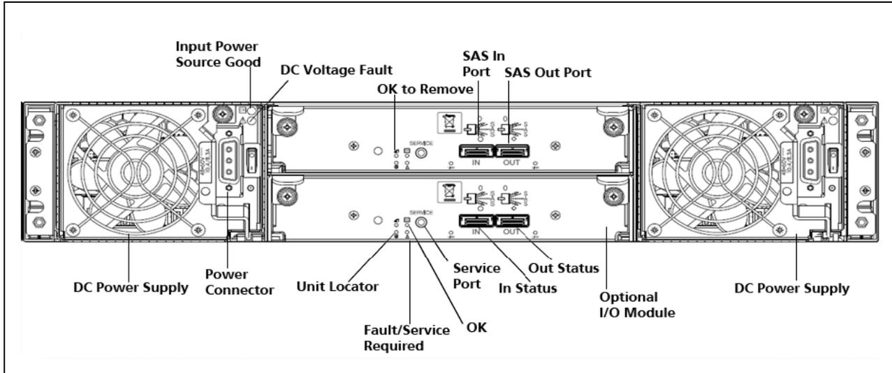
**Figure 4.6 - Expansion Disk Enclosure Rear Panel (DC Power Supplies Shown)**
