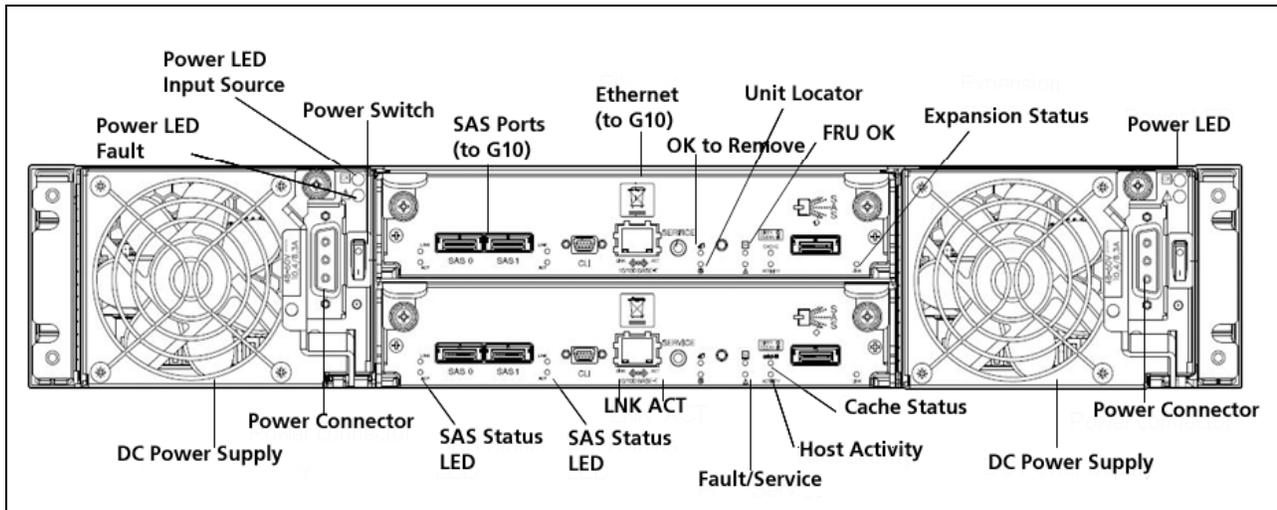
**Figure 4.5 - SA100R Controller Enclosure Rear Panel (DC Power Supplies Shown)**
