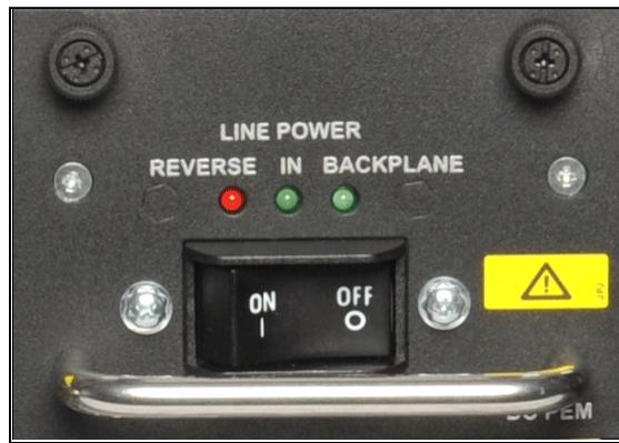
**Figure 2.4 - DC PEM Front Panel LEDs and ON/OFF Switch**
