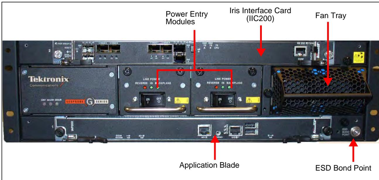
**Figure 1.2 - G10 Probe Front View**
