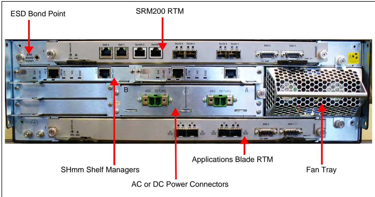
**Figure 1.3 - G10 Probe Rear View**
