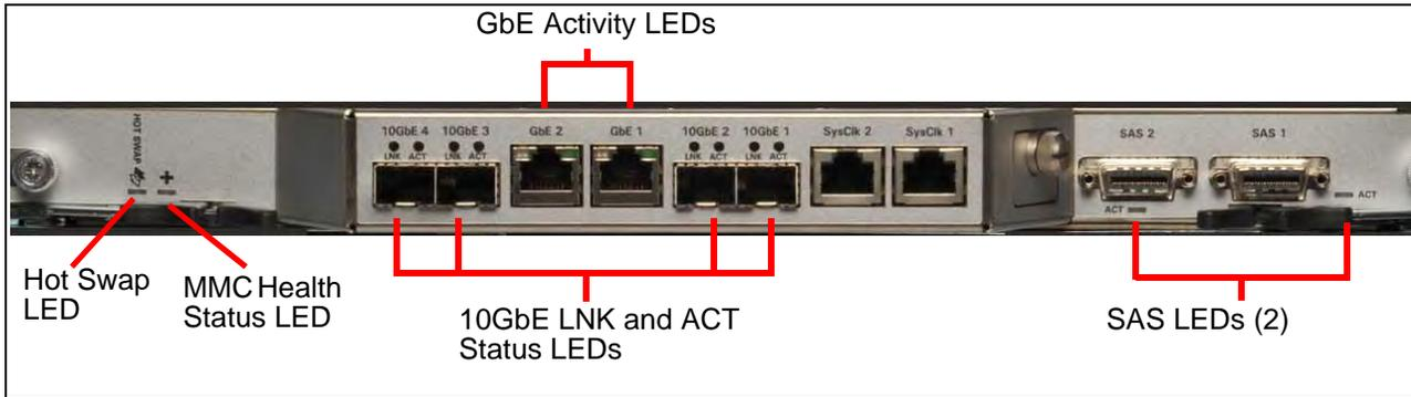
**Figure 3.23 - TRM100 RTM LEDs**
