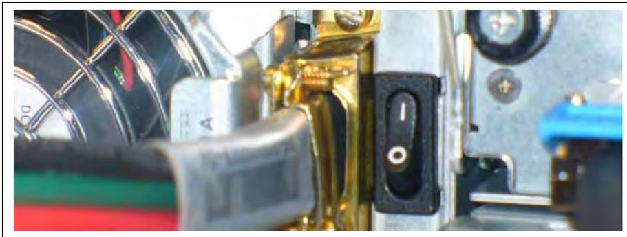
**Figure 5.54 - DC Power Switch on Disk Array**
