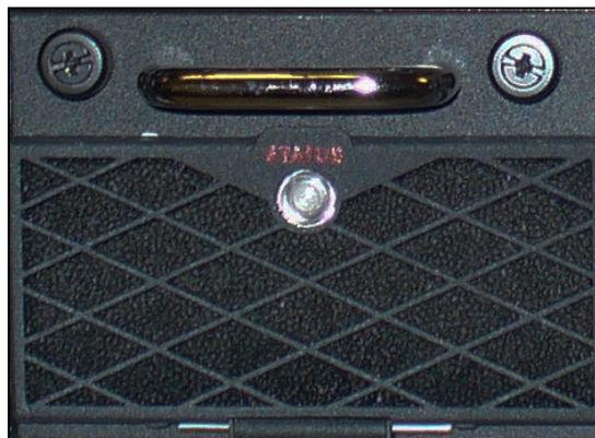
**Figure 2.6 - AC PEM Front Panel LED**
