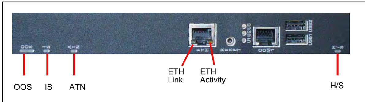
**Figure 3.27 - IAP200 Front Panel LEDs**
