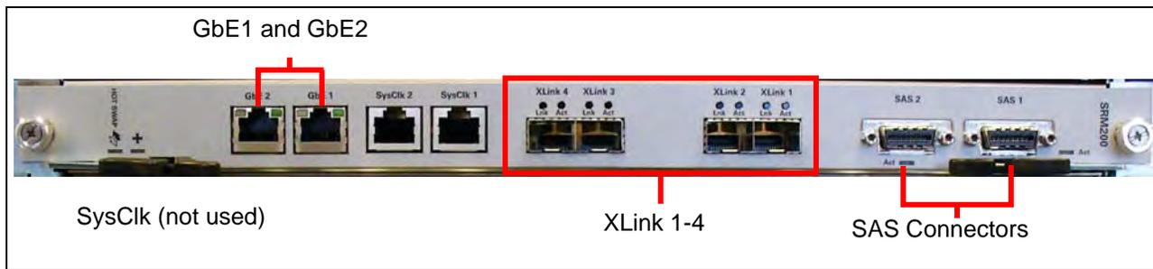
**Figure 3.10 - SRM200 RTM Connectors**
