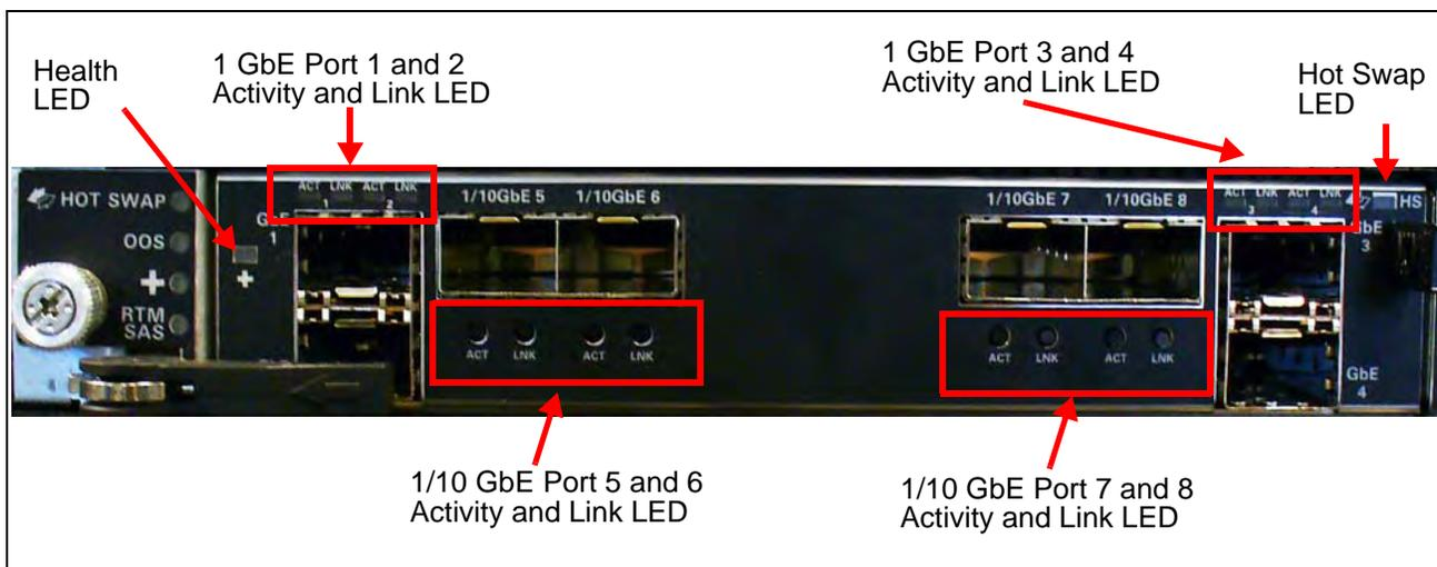
**Figure 3.8 - LPC200 AMC LEDs**
