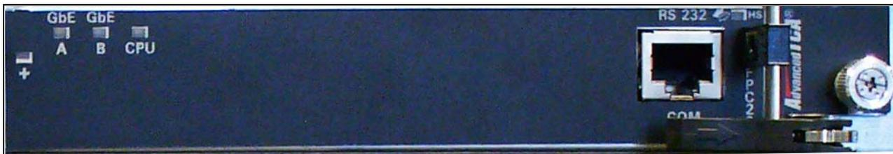
**Figure 3.5 - FPC200 AMC LEDs**
