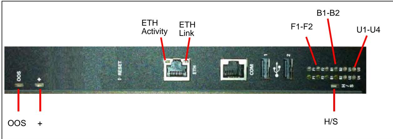
**Figure 3.25 - IAP320 Front Panel LEDs**
