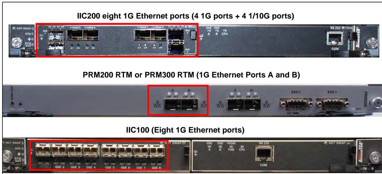
**Figure A.1 - G10 1G Ethernet Connections**
