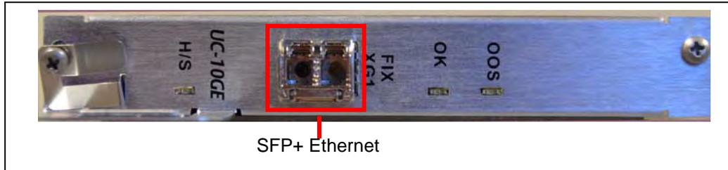
Figure 3.41 - 10G Interconnect Card Connector (Shown with Fiber SFP module)
