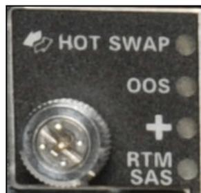
Figure 3.2 - IIC100 or IIC200 Front Panel LEDs
