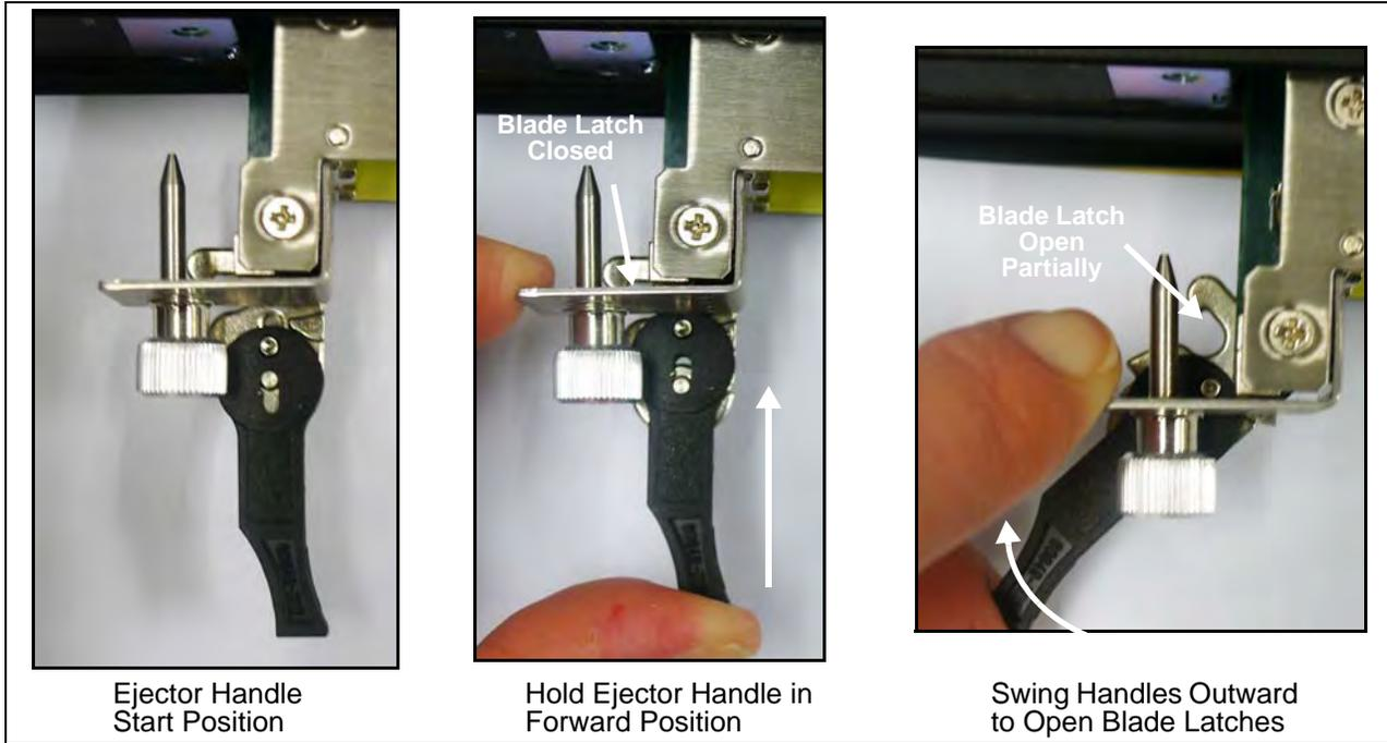
**Figure 5.27 - G10 IIC Ejector Handle (Left) - Opening Blade Latch**
