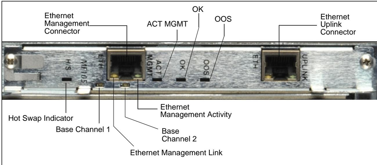
Figure 2.2 - SHmm LEDs
