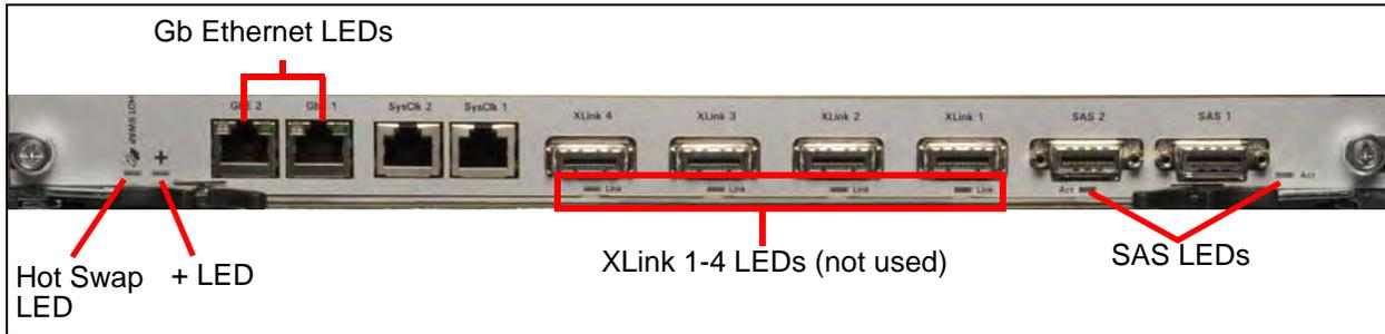
**Figure 3.19 - SRM100 RTM Rear Panel LEDs**
