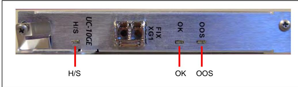
Figure 3.40 - 10G Interconnect Card LEDs
