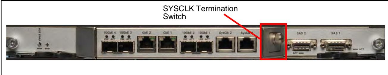
**Figure 3.22 - TRM100 SYSClk Termination Switch**
