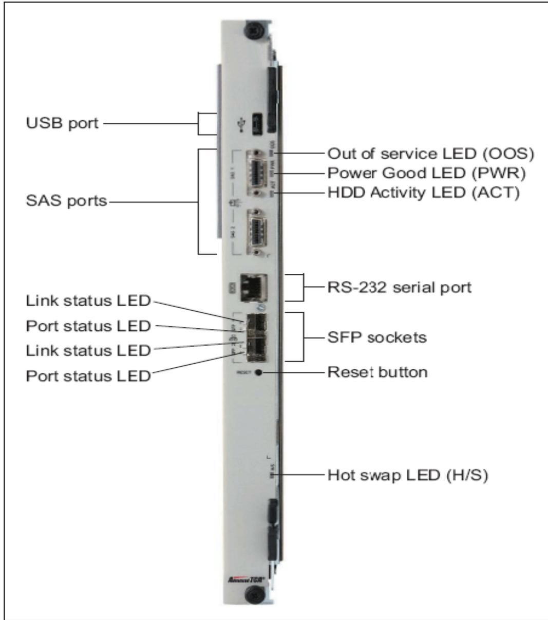
**Figure 3.37 - PRM100 LEDs**
