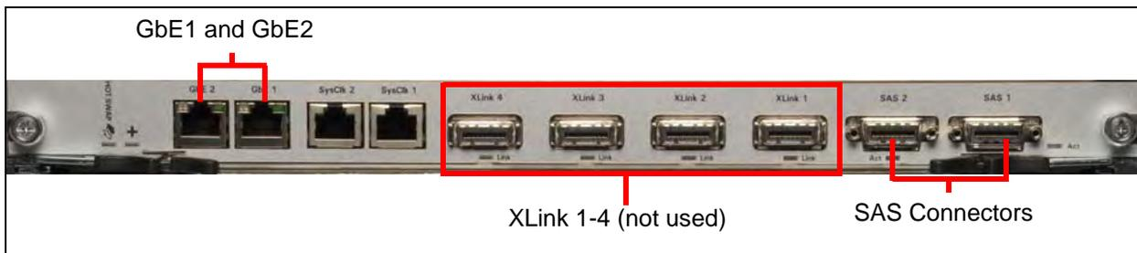
**Figure 3.18 - SRM100 RTM Connectors**
