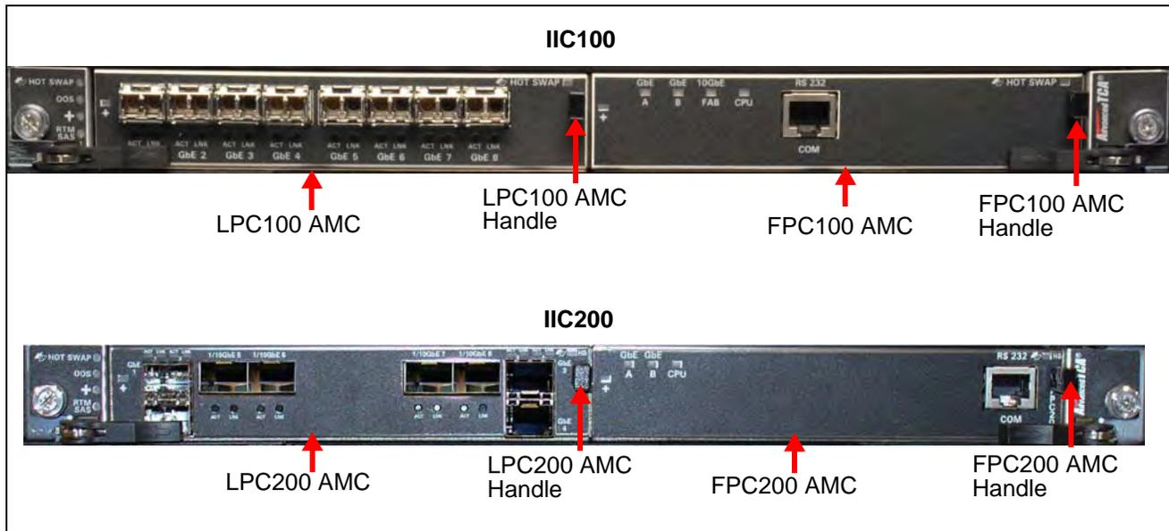
**Figure 5.33 - G10 IIC100 and IIC200 AMCs**
