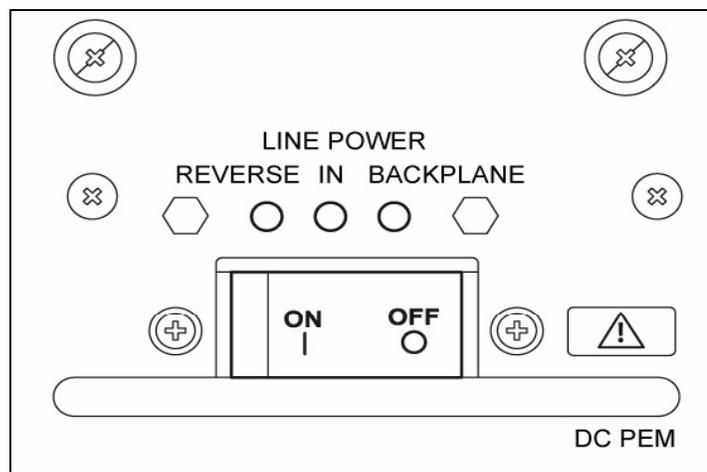
**Figure 6.1 - GeoProbe G10 Power Entry Module (PEM)**
