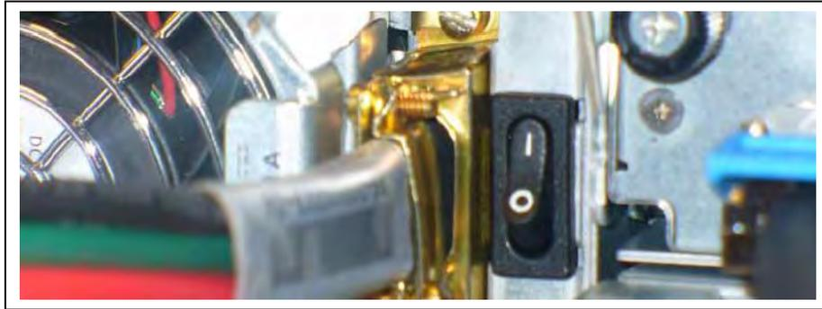
**Figure 5.55 - DC Power Switch on Disk Array**
