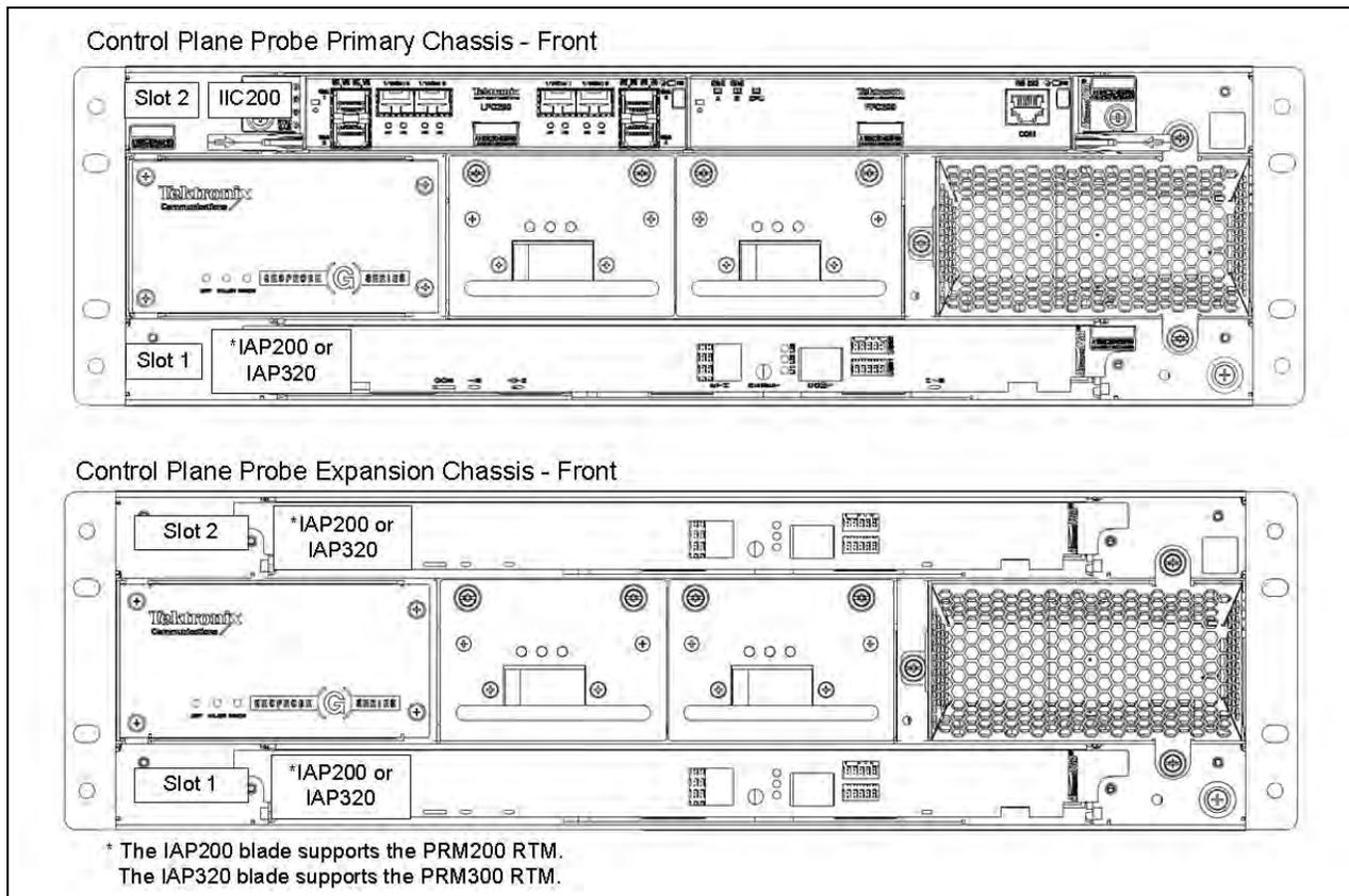
**Figure 1.7 - G10 Control Plane Probe (Front)**
