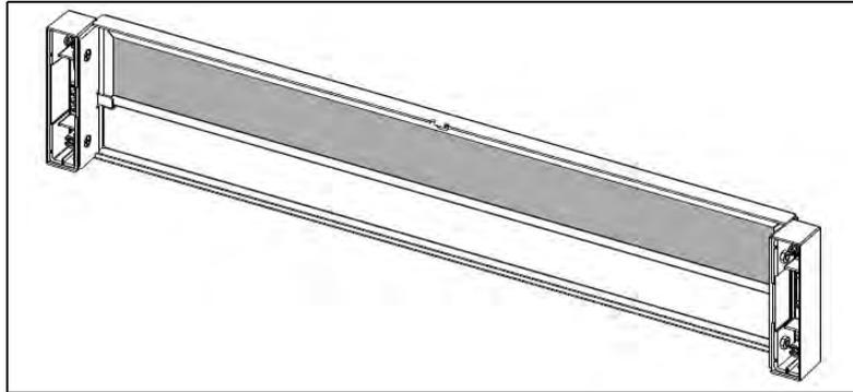
**Figure 5.45 - Air Filter Replacement**
