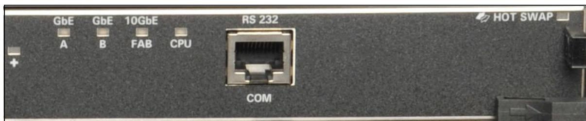
**Figure 3.14 - FPC100 AMC Front Panel LEDs**
