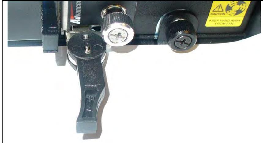
Figure 5.22 - IIC Right Ejector Handle
