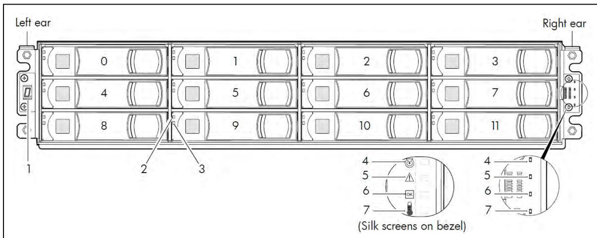
**Figure 4.3 - Near-Line SAS Disk Enclosure Front Panel (SA210J)**
