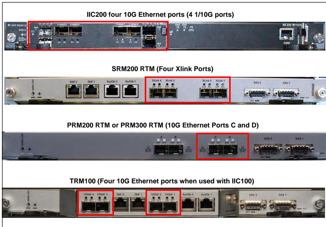
**Figure A.2 - 10 GB Ethernet Ports**
