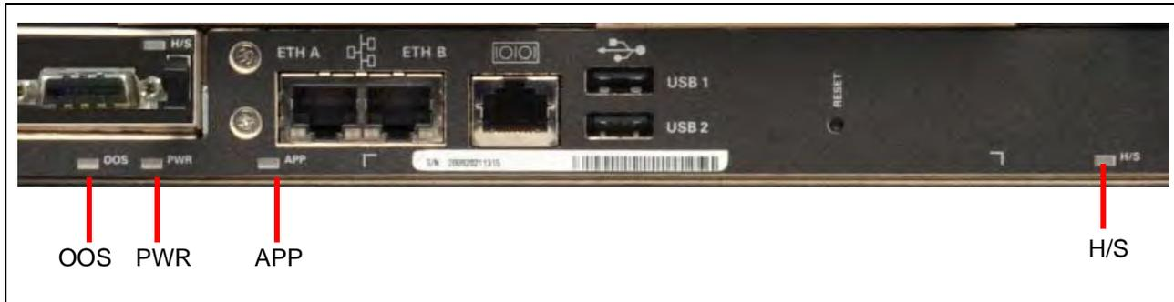
**Figure 3.33 - IAP100 Front Panel LEDs**
