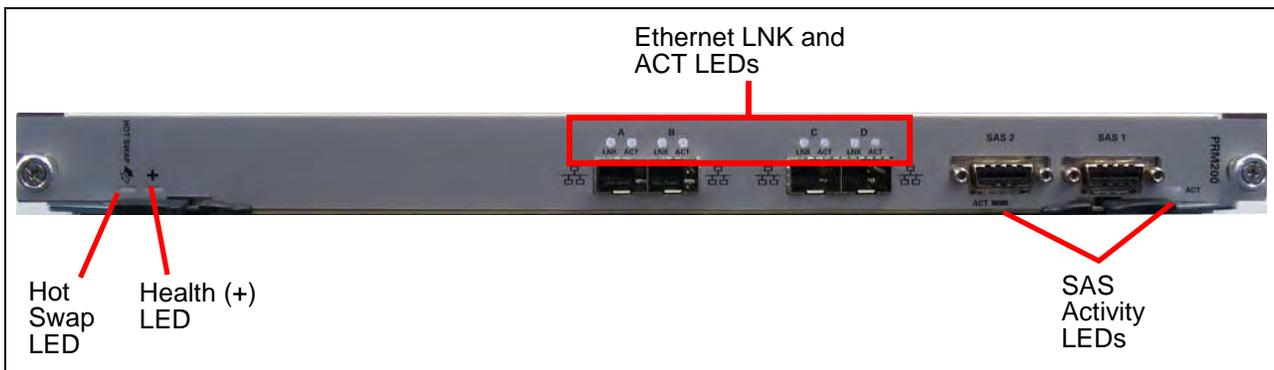
Figure 3.30 - PRM300/PRM200 LEDs
