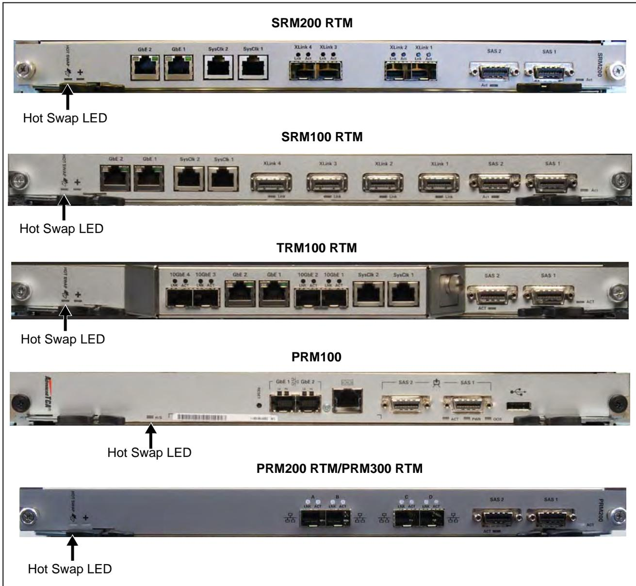
**Figure 5.34 - RTM Hot Swap LEDs**
