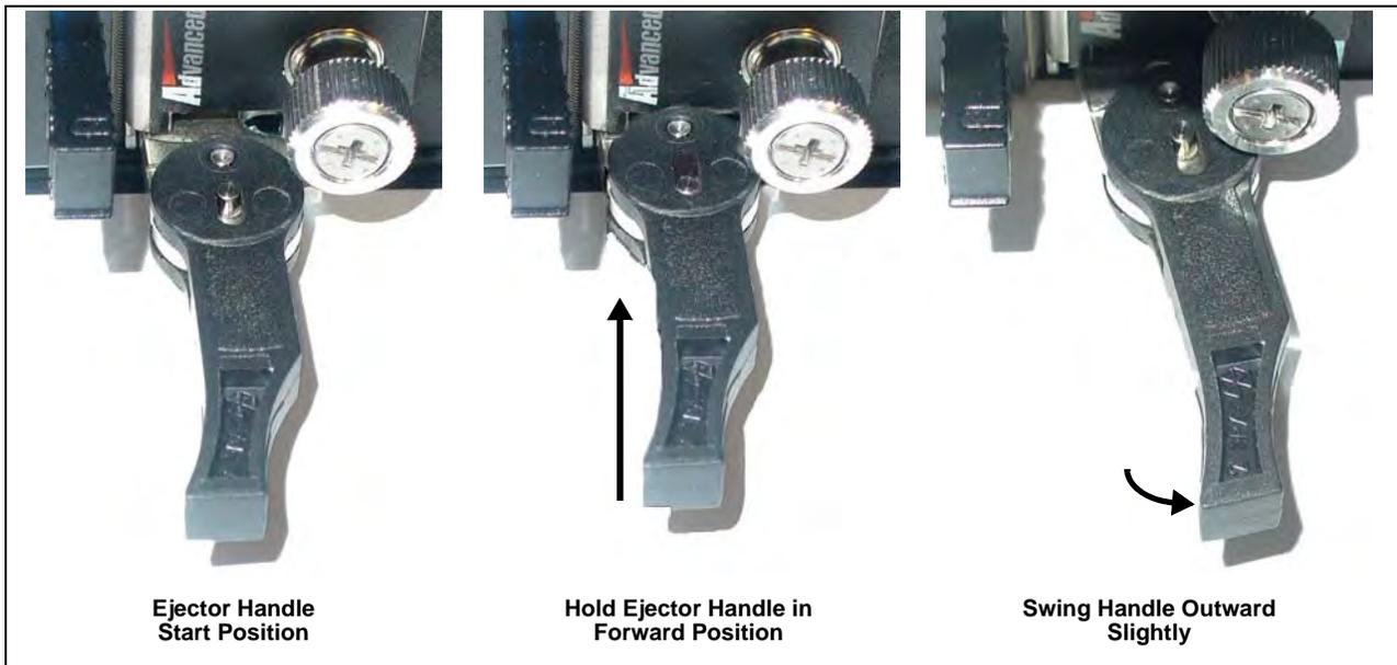
Figure 5.23 - IIC Right Ejector Handle Hot Swap Positioning
