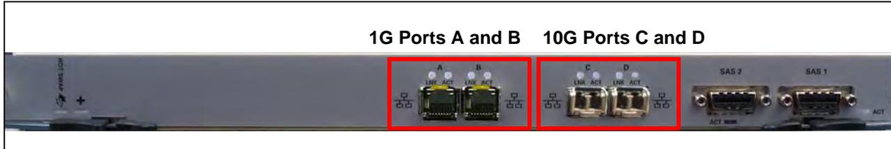
**Figure A.6 - PRM200 RTM or PRM300 RTM SFPs**
