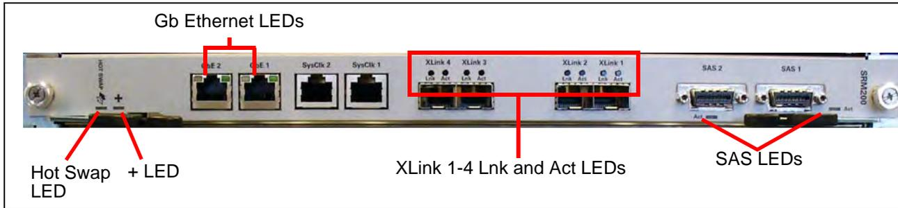
**Figure 3.11 - SRM200 RTM Rear Panel LEDs**
