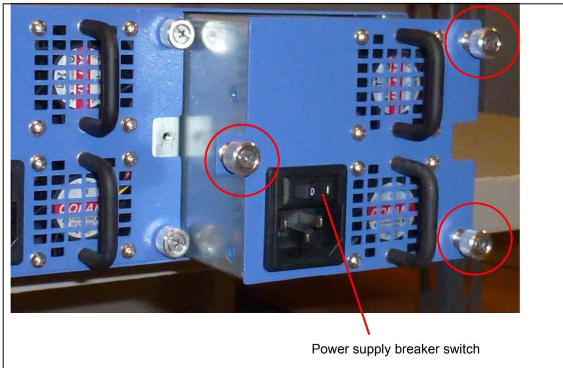
**Figure 6.5 - Loosen Retention Screws**
