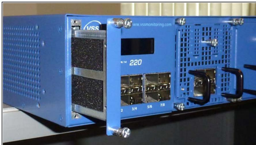
**Figure 6.2 - IPB Chassis Air Filter Removal**
