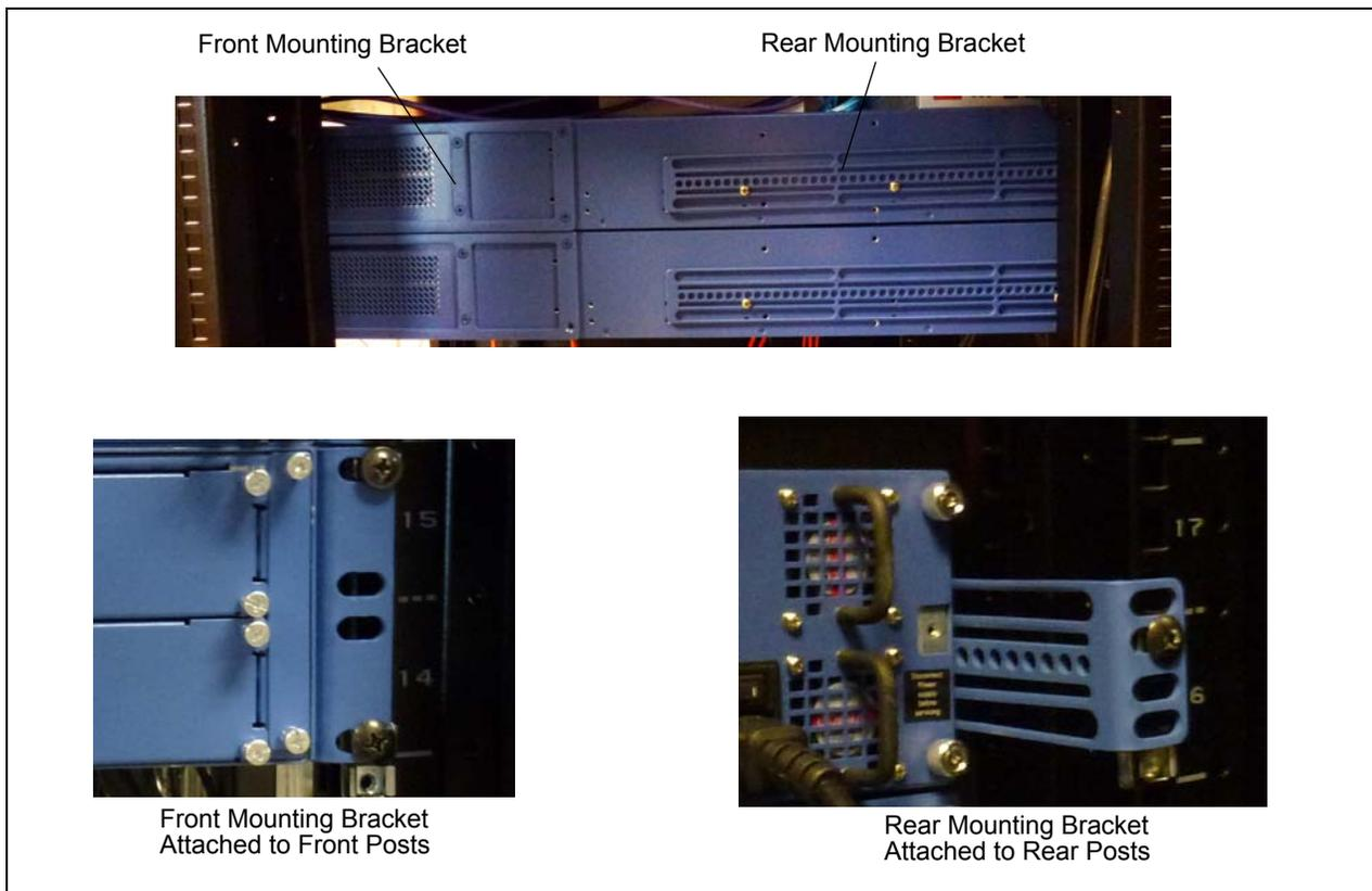
**Figure 3.1 - Installing IPBs (4-Post Rack)**
