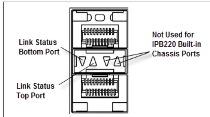
**Figure 2.5 - IPB220 Chassis Port LEDs**
