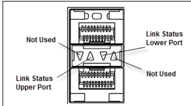
Figure 2.7 - IPB220 and IPB420 1G/10G Chassis Module Port LEDs
