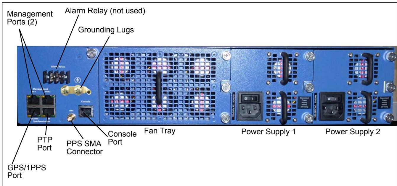
**Figure 2.2 - IPB220 and IPB420 Rear Panel (AC Unit Shown)**
