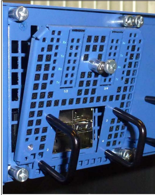
**Figure 6.4 - IPB Chassis Air Filter Removal**
