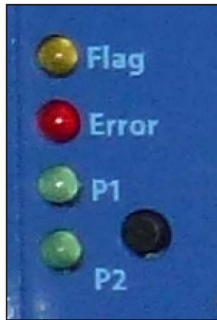
**Figure 2.3 - IPB Chassis LEDs**
