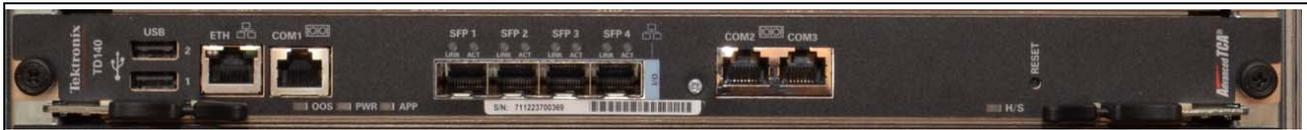
**Figure 3.3 - TD140 PPM40 Blade**
